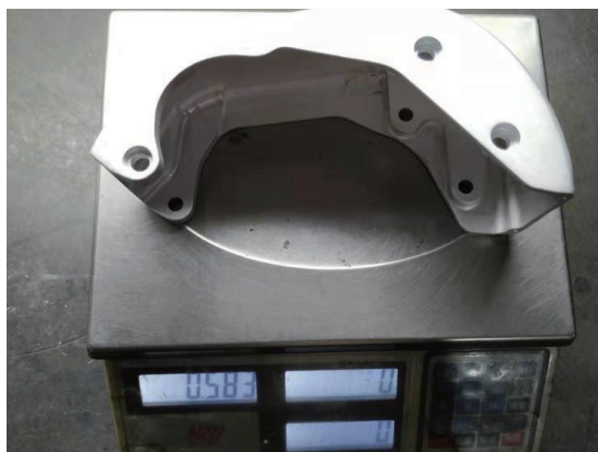
▲ Traditional one-piece forged motor bracket. Weight: 583g
