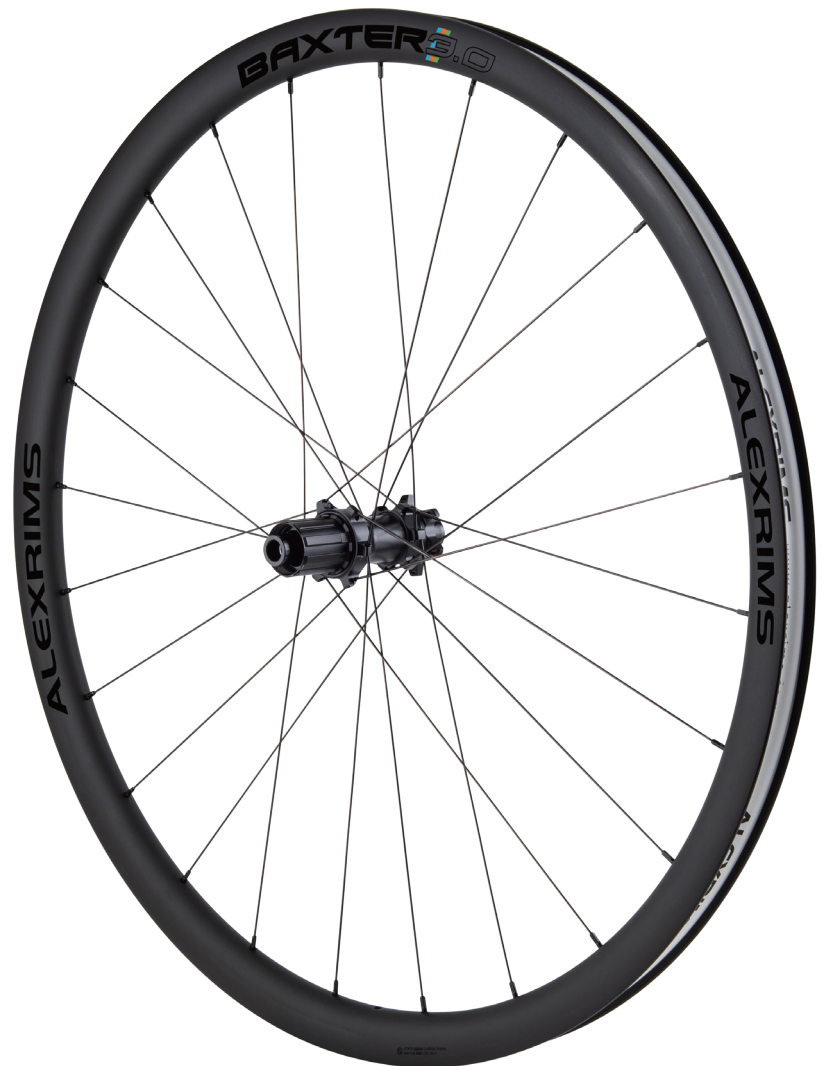
▲ Baxter 3.0 wheels designed for gravel bikes.
