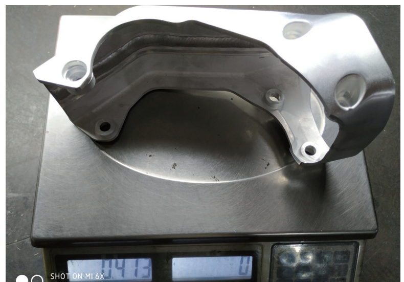
▲ New two-piece welded motor bracket. Weight: 413g
